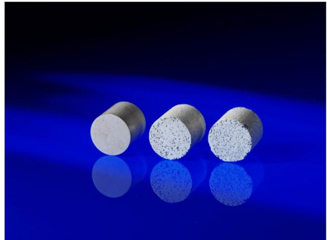
Fig. 3. Hydroxyapatite / PLA composite with different grades of porosity (increasing from 0% over 20% to 50% from left to right) for potential application as bone replacement material (IFAM).
