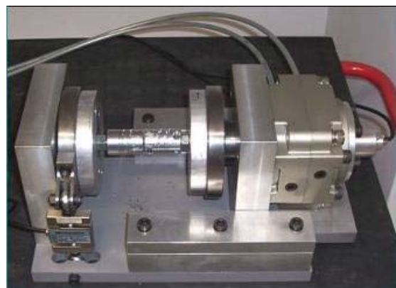
Fig. 2. Torsion machine to measure shear strength (POLITO)
